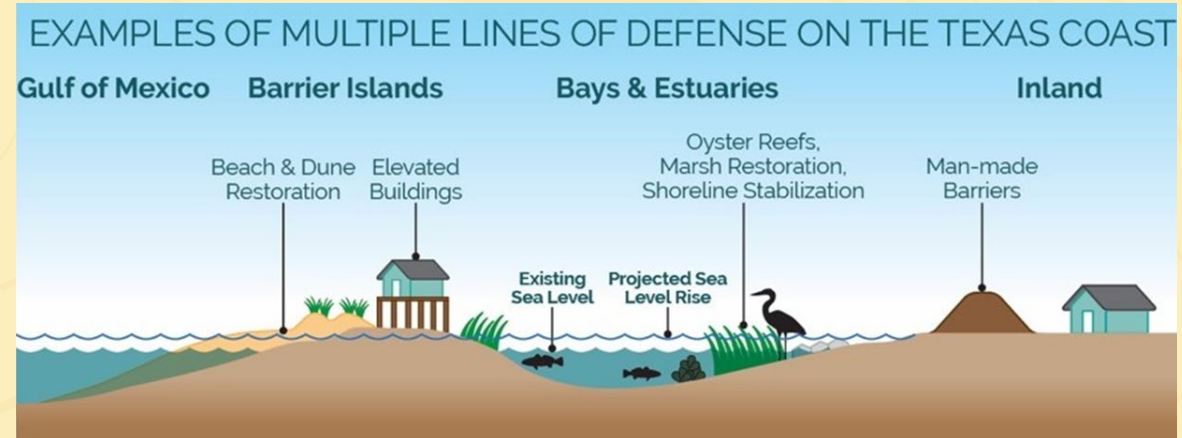
Figure 2-10. Multiple lines of defense on the Texas Coast Source: The General Land Office
