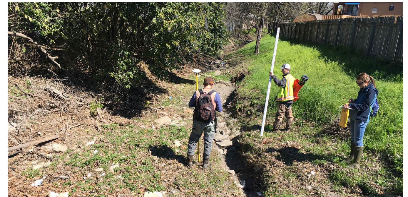
Figure 10-2. Turtle Creek in Austin, Texas. This is an example of a Class III channel. The image shows the degradation associated with an unstable, sediment limited stream.
